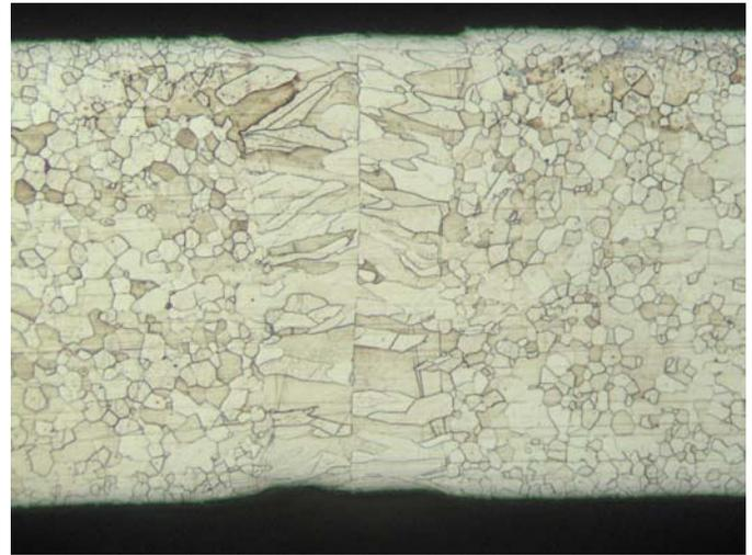
*Figure 6: Laser Welded Stainless Steel Tube Weld Pattern*
