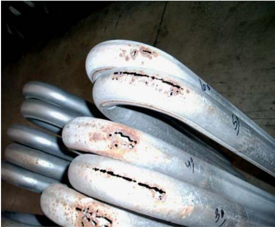
*Figure 2: Corroded Aluminized Steel Heat Exchanger*
