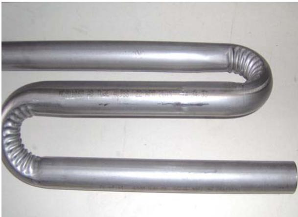
*Figure 13: Serpentine Wrinkle-bent tube*
