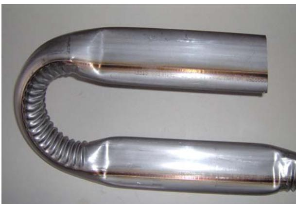
*Figure 14: Wrinkle-bent and flattened tube*
