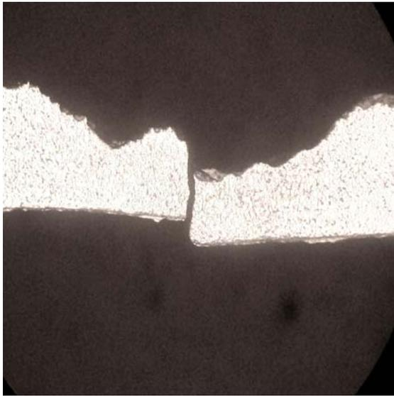
*Figure 4: Oxidized Aluminized Steel I.D. Tube Weld Cross-section*
