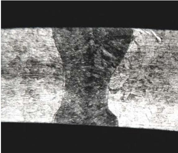
*Figure 5: TIG Stainless Steel Tube Weld Pattern*
