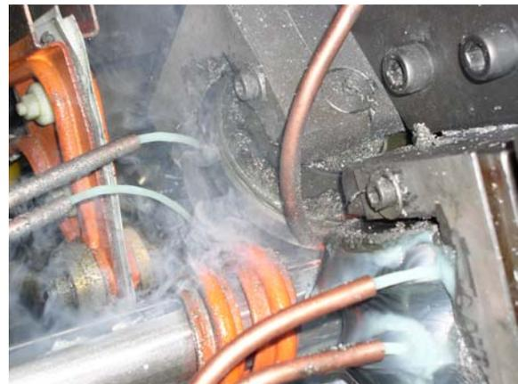
*Figure 9: UHFSS Coil and Weld Box Area*
