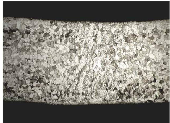
*Figure 10: Typical UHFSS 409 SS Tube Weld Zone/HAZ*
