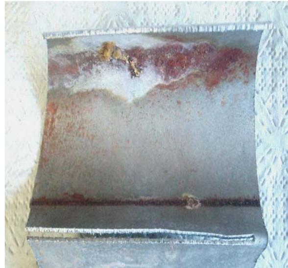
*Figure 3: Oxidized Aluminized Steel Tube I.D. Section*
