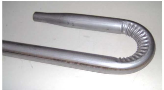
*Figure 15: Wrinkle-bent and "pointed" U-bend tube*
