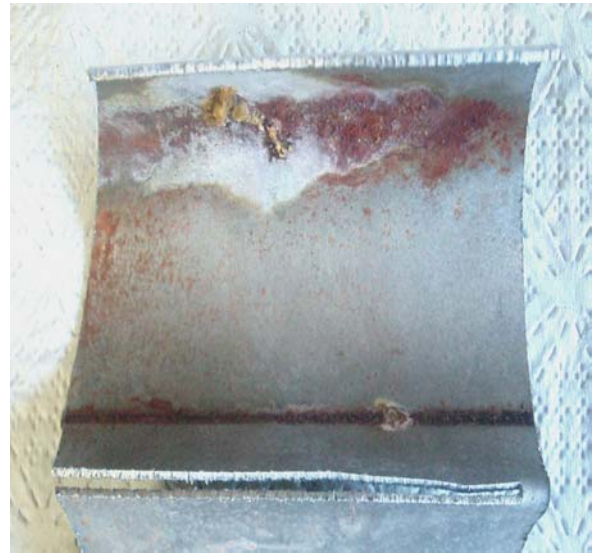
Figure 3: Oxidized Aluminized Steel Tube I.D. Section
