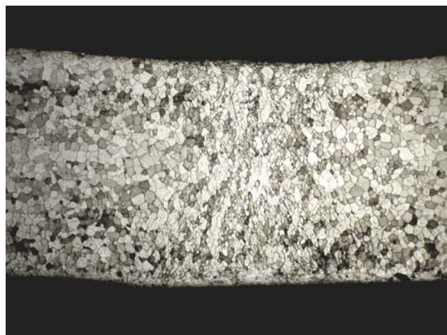
Figure 10: Typical UHFSS 409 SS Tube Weld Zone/HAZ
