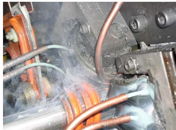
Figure 9: UHFSS Coil and Weld Box Area
