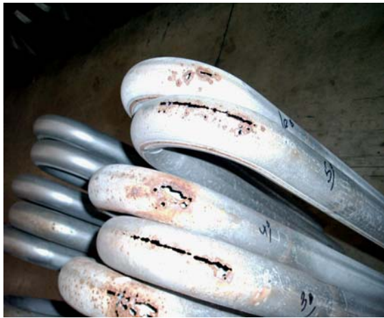
Figure 2: Corroded Aluminized Steel Heat Exchanger
